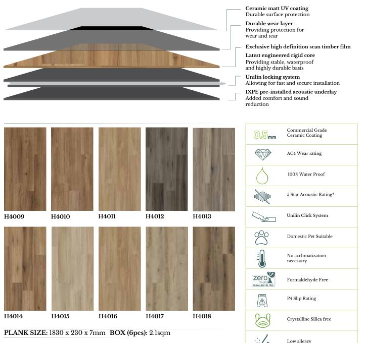
Installation guidelines provided on request. We recommend 8mm expansion gaps to walls, cabinetry & fixed furnishings. Suitable for underfloor heating up to 35° \* Acoustic rating subject to installation.
